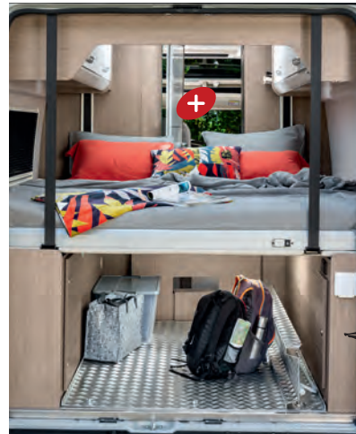
+ Daytime position : The (electric) fold-down bed lies flat against the ceiling or in its intermediate position, freeing up a large living space and/or storage space Night position: In its low position, the bed becomes extra large: 190 x 190 cm
