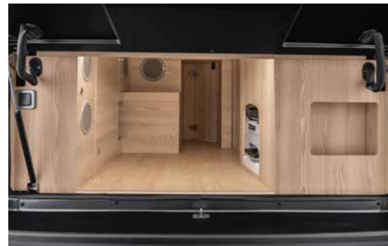
Access to the boot, toilet cassette and external shower is possible by lifting the flap at the rear of the vehicle.
